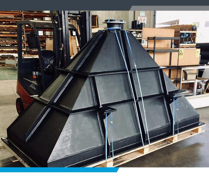
Industrial Plastics can process the design and fabrication of HDPE hoppers for sophisticated projects primarily in the mining and resources sector. The hoppers separate material into a specific section at the bottom. Our sales team will engage with customers about their product specifications to create a successful product to be delivered anywhere in Australia.
