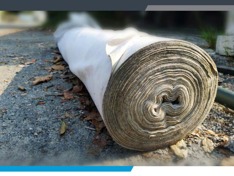
Geotextiles provide filtration, drainage and separation of engineering materials in a variety of construction structures associated with transportation and infrastructure activities. Geotextile materials, when selected appropriately, allow for the replacement of traditional granular filter and drainage layers, providing a significant environmental and economic benefit. The use of geotextiles has gained tremendous acceptance over the last 30 years.
