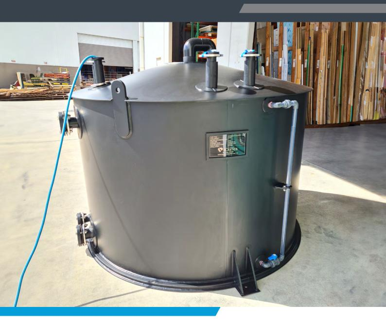
We fabricate dual walled sodium hypochlorite tanks with a design life of 25 years. The twin wall design provides extra safety in the event of a tank failure, which prevents the release of bulk hazardous material. This feature makes it one of the safest options on the market while also increasing its design life. Industrial Plastics use PVC because of its resistance to chemical oxidising, which is required when storing bleach.
