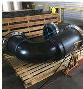
All of our pipework is fabricated to DVS 2007 and ISO 9001: 2015 standards to maximise product performance and ensure that our products exceed our market leading quality guarantee. All pipework is rigorously tested using various methods including pressure testing, spark testing and hydro testing before delivery to site. We have in house pressure and hydrostatic testing capabilties as well as MDR's, all certified to ISO 9001: 2015.
